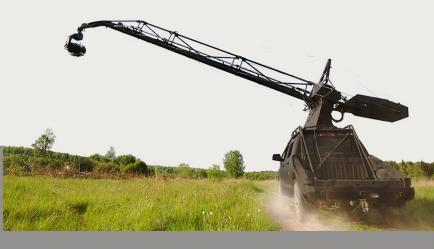
gigantic, weighing more than 85kg. Light and agile "Black Unicorn Crane" allows shooting at a carrier speed of over 180 km/h and 90 km/h off-road. Remote control of the crane is realized from the cabin of the vehicle. Crane is not difficult to uninstall from the roof of the car and to install on other types of vehicles, for example, on a boat or a train.
